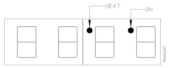
d. Verify that motors heat, and door indicator lights on the back side of the microprocessor (computer board are lit. (Refer to illustration below.)
